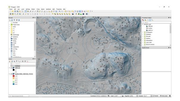
It is evident that the labelling is not optimal. By default each individual loop of a contour is labelled which, for example, yields a large number of 1-m labels in the irregular micro-topography in the lower left corner of the map. For the purpose of what we want to achieve, to investigate topography, we can live with this. With time during your education you will learn how to make maps that are nicely formatted so this is just a start.
