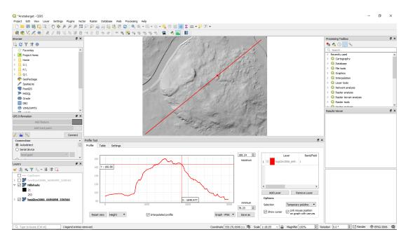
Note that the profile in the graph window is plotted from left to right as you started and stopped your profile. In this case I started the profile in the lower left corner and finished in the upper right corner so that the plotted profile depicts the general direction of the profile in the map.
