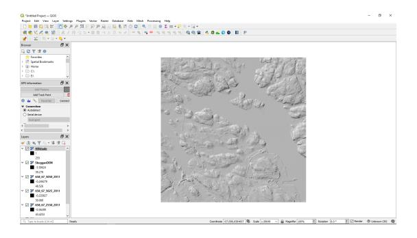
At this point it is worth noting that in the lower left of the QGIS window you see two entries, the elevation data file 'SkugganDEM' and the 'Hillshade'. These are layers. The reason the Hillshade is shown is because this layer is on top of the DEM. You can turn the Hillshade on and off by checking and unchecking the Hillshade layer. You can also reorder the layers by dragging and dropping the layers in the order you want them. For now the original order makes most sense.
