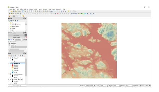
What you see now is that the elevation data goes from red at low elevations to blue at high elevations and that the shaded relief effect is still there but 50% translucent to show the coloured DEM. This indicates how you can work with the layers to create a good end product that gives the viewer information on elevation and relief.
