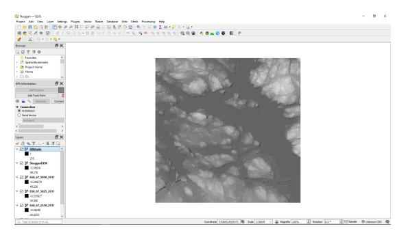
We can also modify the DEM layer. Let us add some colour to it by 'right-clicking' on the elevation layer. This opens the Layer properties dialog for the layer. Select the 'Style' option by clicking on it.
